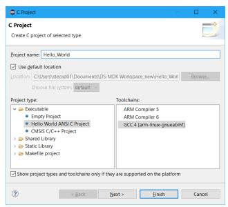
Enter a project name (for example **Hello\_World**) and make sure that the **GCC** [...] (built-in) toolchain is selected before clicking **Finish**.
