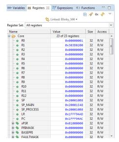
The search button at the top of the View allows searching for register by name to speed up debugging in targets with hundreds or thousands of different registers.
