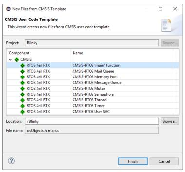
Expand the software component **CMSIS** and select the template **CMSIS-RTOS** 'main' function. Click **Finish**. Replace the content of *main.c* with the following application specific code:
