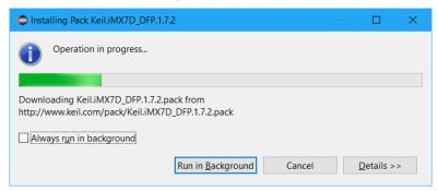
At the end of the installation the CMSIS Packs for the selected board should be installed locally and the examples are ready to be copied in your workspace.
