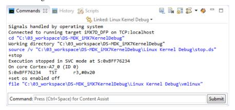
In the Command (CLI) entry box, set a temporary hardware breakpoint (thbreak) on the entry point into the kernel, by typing in:
