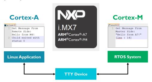
The *Linux Application TTY* runs on the Cortex-A processor and writes a message to a TTY device. The terminal of the *RPMSG TTY RTX* application running on the Cortex-M processor shows this message. The application itself responds on the TTY device. The Linux application reads this message and shows it in its **App Console**.
