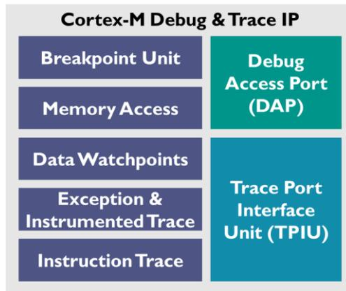
The **Trace Port Interface Unit (TPIU)** is available on most Cortex-M3, Cortex-M4, and Cortex-M7 processor-based microcontrollers and outputs above trace information via:
