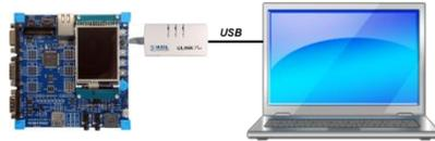
CMSIS-DAP based USB JTAG/SWD debug interfaces are typically part of an evaluation board or starter kit and offer integrated debug features. MDK also supports several proprietary interfaces that offer a similar technology.
