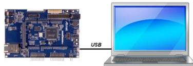
MDK connects to third-party debug solutions such as Segger J-Link or J-Trace. Some starter kit boards provide the J-Link Lite technology as an on-board solution.
