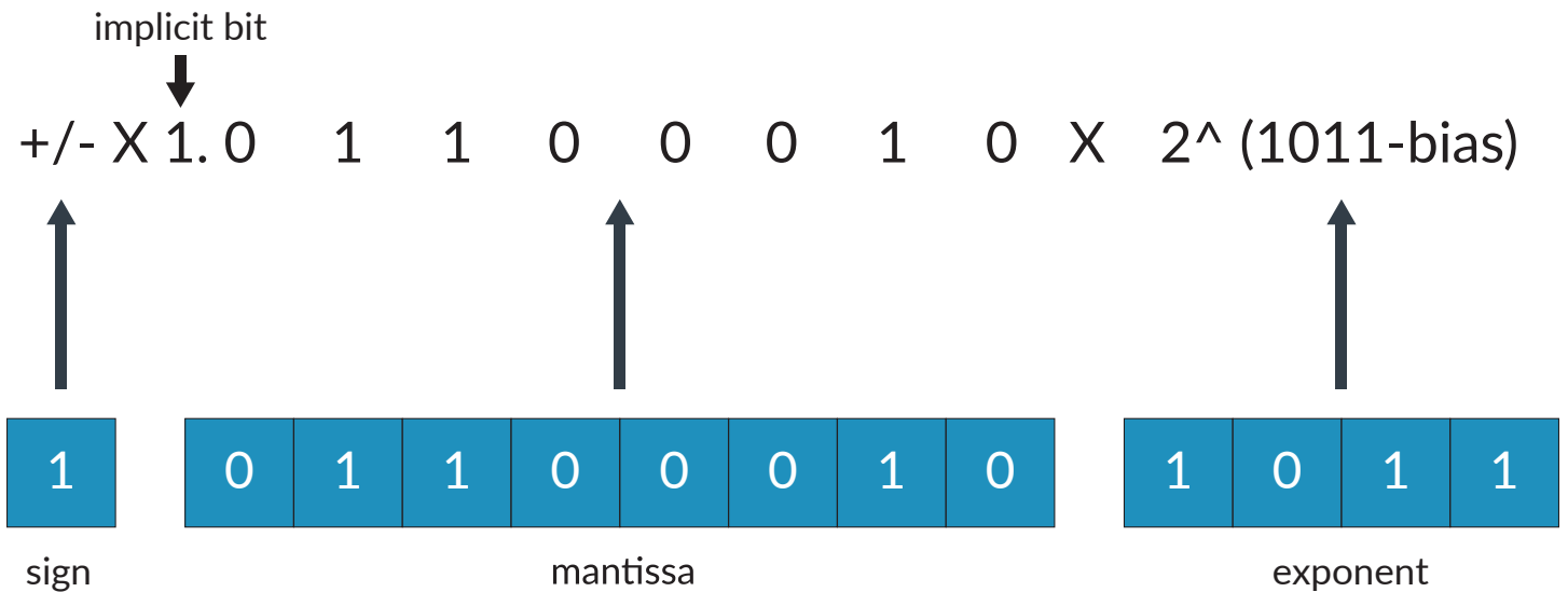
Figure 2. Floating-Point Representation of Scale Factor
