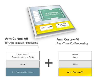
The Arm Cortex-A9 hard processor in the Zynq FPGA can run compute-intensive and application tasks; whereas the Cortex-M can be utilized for real-time tasks such as industrial automation, motor control, etc. While the Cortex-A9 can have a rich operating system such as Linux; the Cortex-M can run a RTOS for bounded interrupt latency.
