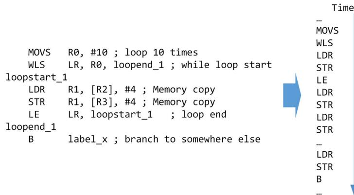
The first time the loop is executed, both WLS and LE instructions would be executed, and the loop addresses are cached inside the processor, and subsequent loop iterations do not need to execute these two instructions again. The loop counting is handled by the link register (LR/r14) and the loop exit, when the loop counter reaches zero.
