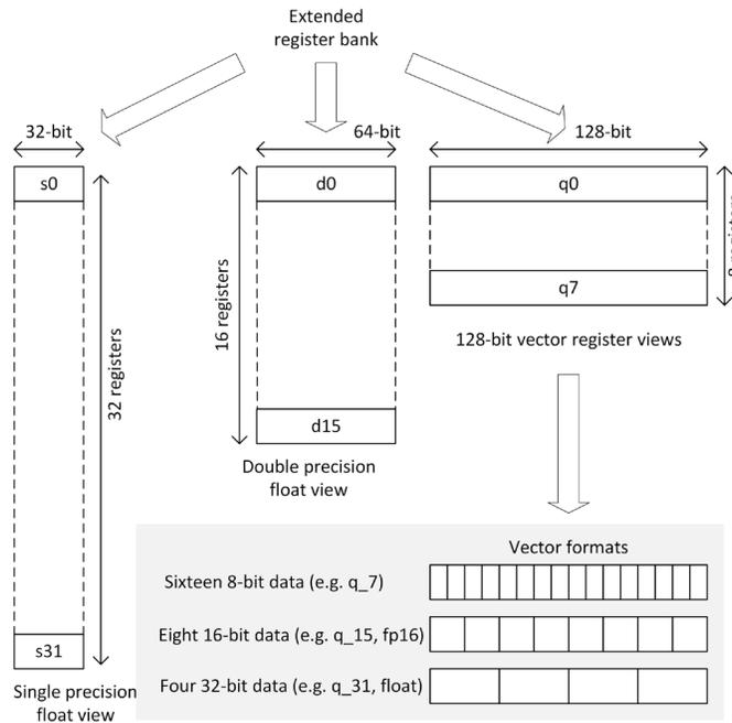
The integer support in Helium enables efficient compute of 8-bit, 16-bit and 32-bit fixed point data. 16-bit and 32-bit fixed point formats are widely used in traditional signal processing applications, such as audio processing. 8-bit fixed point format can be important to machine learning (ML) processing, such as neural network computation, as well as image processing.
