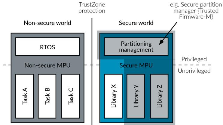
With the unprivileged debug extension, debug access to memory of current security state (except certain debug components inside the processor) is blocked when the processor is running and is allowed when the processor is halted in the unprivileged state, with unprivileged debug enabled (UIDEN bit in DAUTHCTRL set to 1). The debug accesses also check against the permission in the MPU of the current state, when unprivileged debug is used for that state.
