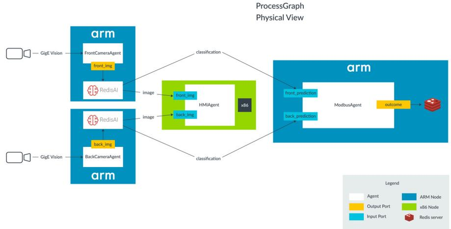
All the agents run in Docker containers. Each node capturing images from the cameras run two containers, one for the camera agent, and one running Redis. Similarly, the node running classification agents runs two containers, one for front image classification, and one for the back.
