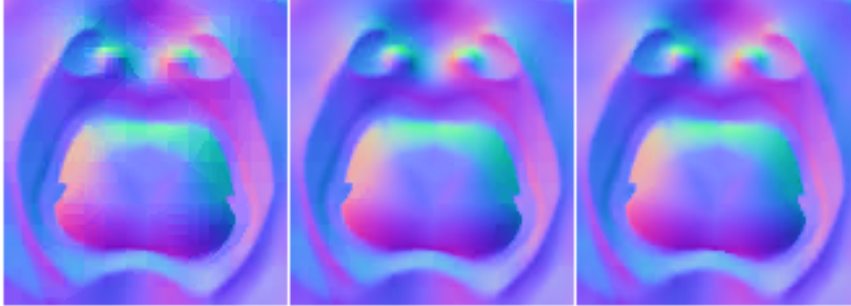
Figure 1.5. The leftmost normal map is compressed with default settings, the second uses normal_psnr and the normal map on the right uses -normal_percep
