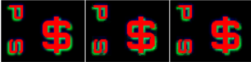
Figure 1.6. The left image is the uncompressed data, the second is compressed with default settings, the right image uses the mask argument.
