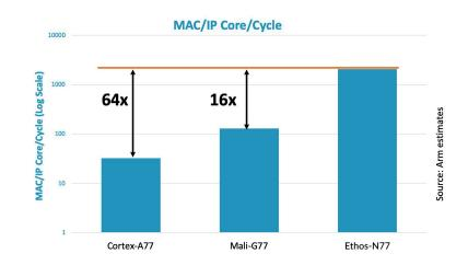
Ethos-N77 delivers single-core performance of < 4 TOP/s with efficiency of < 5 TOPs/W
