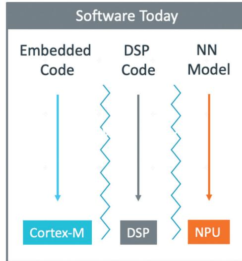
Ethos-U55 and Cortex-M55 provide an opportunity to run this code on a single toolchain. The following features help reduce complexity and eases software development:
