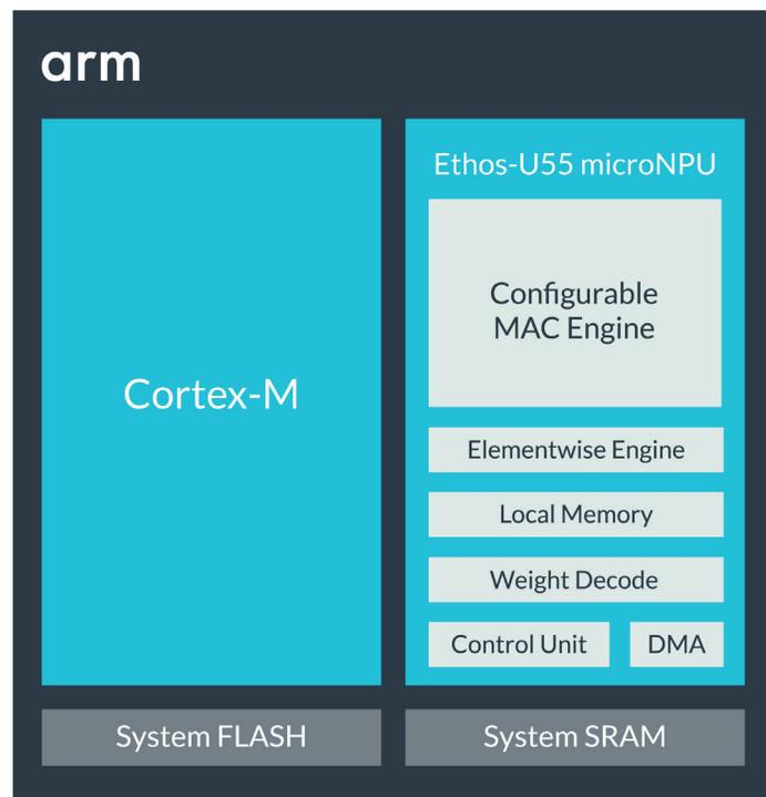
Ethos-U55 accelerates a fixed set of high compute operators in hardware. Other operators run on the attached microcontroller. It is the easiest way to add more neural network acceleration capability to Cortex-M based systems in a very small silicon area cost. The smallest version of the IP can fit in approximately  $0.1\text{mm}^2$  area in 16nm process.
