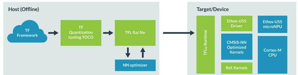
The process starts by training or acquiring a TensorFlow model that is to be accelerated. The model is then quantized to 8-bit integer format and converted to the standard TensorFlow Lite flat file format. The NN optimizer tool, provided by Arm, reads this TensorFlow Lite flat file as an input and formats it to make it ready for deployment.
