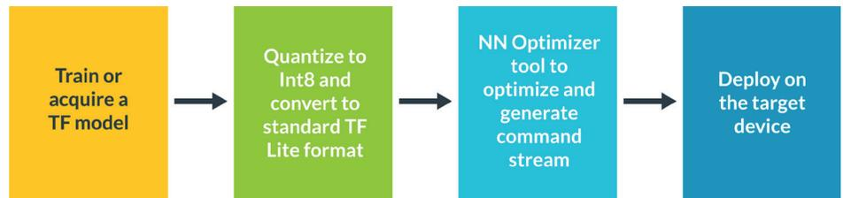
Arm is working on developing TensorFlow Lite Micro in an open source collaboration with Google to help accelerate neural networks in an extremely small memory footprint. TensorFlow Lite Micro doesn't require operating system support, standard C or C++ libraries, or dynamic memory allocation. The core runtime fits in 16KB on a Cortex-M3 processor, and with enough operators to run a speech keyword detection model, takes up a total of 22KB.<sup>[1]</sup>
