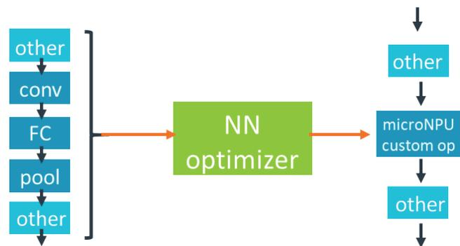
After reading the flat file, the tool identifies the subgraphs that can execute on the Ethos-U55 microNPU and optimizes the scheduling of these subgraphs. Several factors are taken into consideration for this optimization:
