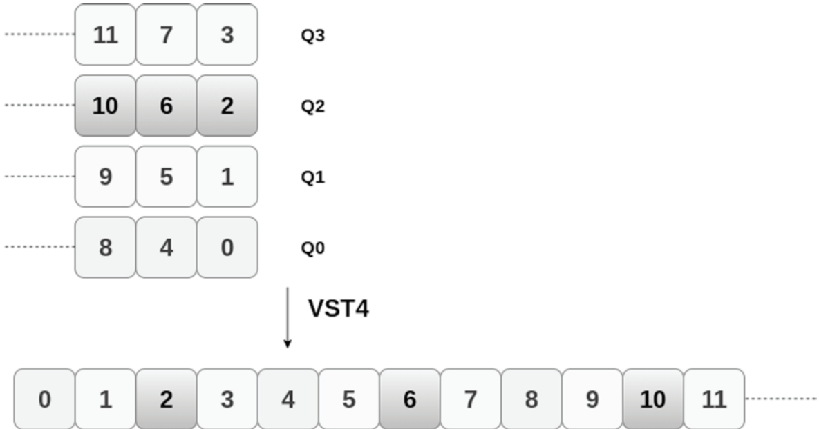
Figure 5.5: Interleaving of pixel data using VST4
