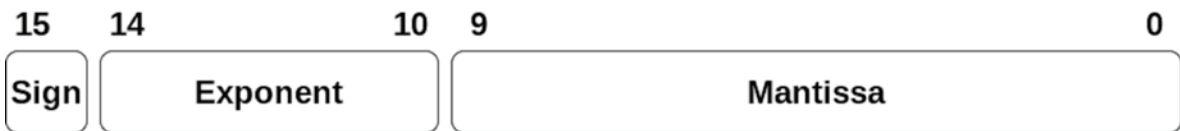
Figure 2.2: Half-precision floating-point number format
