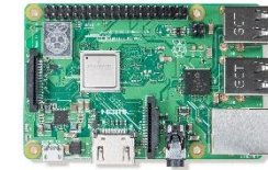
Raspberry Pi B+ - Cortex A53, 2MB L2, 1GB DRAM, 1.2GHz
